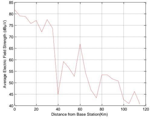
Figure 2: Signal Propagation Curve for Yenagoa-Ughelli Route
